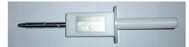
Lengthened test finger
