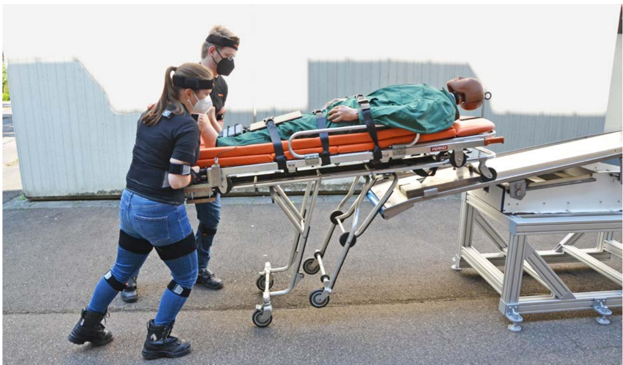
Two test persons pushing a mechanical wheeled stretcher up onto the stretcher platform.
