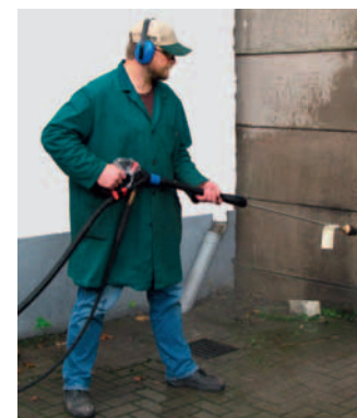
Measuring the vibration on the spray gun of a high-pressure cleaner
