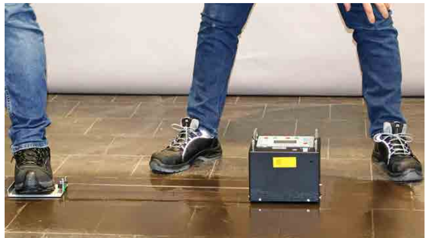
In-situ testing using a GMG 200 mobile tribometer on sliders fitted with a range of footwear materials
