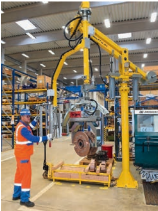
Inclusive workplace design: workpiece manipulator on a lathe
