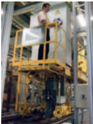
Fixed servicing access point (platform) on a machine
