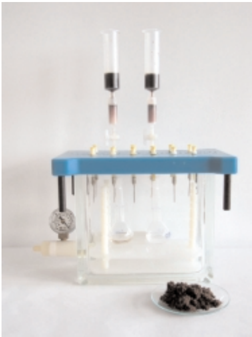
Prior to chromate measurement according to CEN, unwanted colourants are removed from the eluate obtained from the sample.
