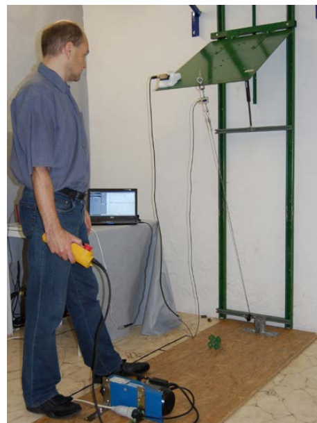
Fig. 139: Closing of a flap. Measurement apparatus with winch (automated speed, pulling force sensor and angle measurement, and integral gas spring)
