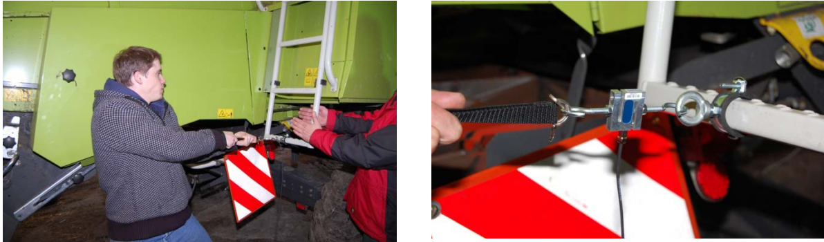
Fig. 122 and Fig. 123: Disengaging the ladder to the grain tank, combine harvester (Claas Mega 350). Measurement by means of a transducer, fixing of the force application point by means of a hose clip, test subject 2 (left), test subject 3 (right)
