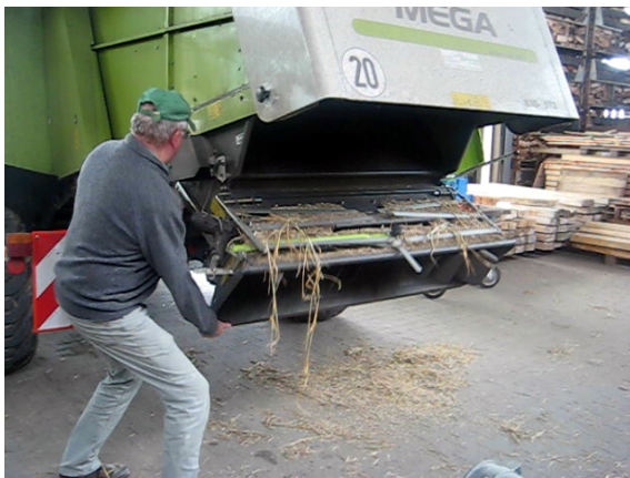
Fig. 25: Manual chopper adjustment on a combine harvester (Claas Mega 350). This form of manual chopper adjustment is frequently found on smaller combine harvesters
