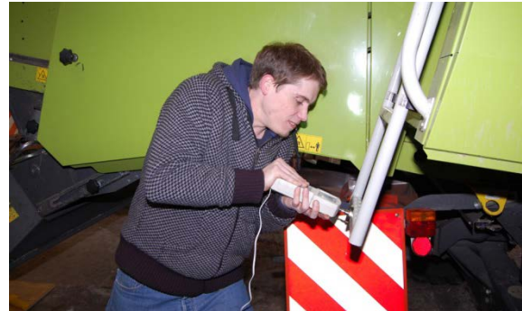
Fig. 115: Measurement with a hand-held force meter, fixing of the force application point by means of a magnet, test subject 2
