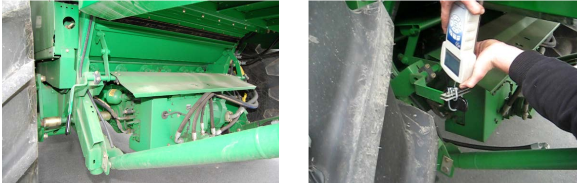
Fig. 82 and Fig. 83: Lever on the inclined conveyor of a combine harvester (John Deere T560). Measurement of the pulling force by means of a hand-held force meter; force transmission by means of a hose clip; test subject 2
