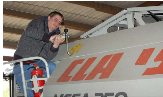
Fig. 76 and Fig. 77: Opening of a grain tank on a combine harvester (Claas Mega 350). Half a turn is required to open the tank. Measurement by means of a hand-held force meter. Left: test subject 1; right: test subject 2
