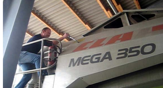
Fig. 12: Opening of a grain tank on a combine harvester (Claas Mega 350); half a turn is required to open the tank
