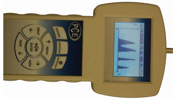
Fig. 5: Example of a hand-held electronic force meter: PCE-FG 500. Saving of force/time characteristics is possible
