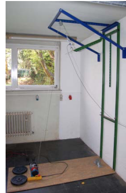
Fig. 7: The force measurement system shown in Fig. 6 fitted on the measurement apparatus, with additional automatic speed control provided by a winch
