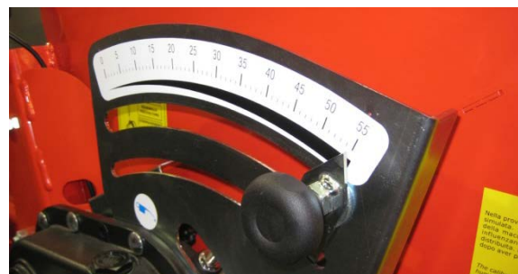
Fig. 36: Angle adjustment with locking screw
