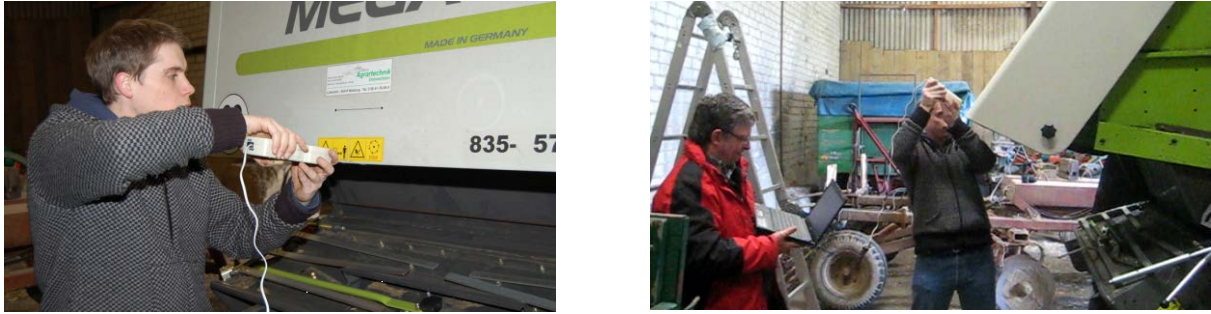
Fig. 85 and Fig. 86: Opening of a rear flap on a combine harvester (Claas Mega 350), measurement with hand-held force meter, test subject 2
