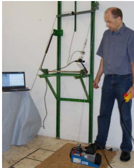
Fig. 133: Operation of a lever. Measurement assembly with winch (automated speed, strain sensor and angle measurement)
