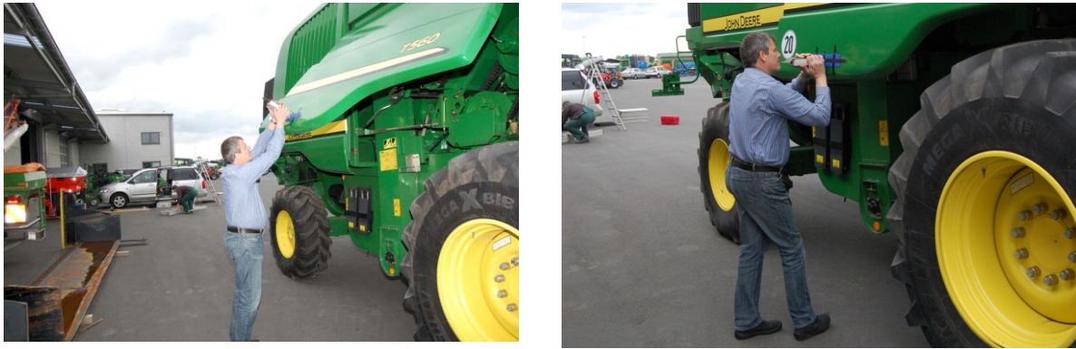
Fig. 97 and Fig. 98: Closing of the right-hand side flap on a combine harvester (John Deere T560): measurement of the pushing force by means of a hand-held force meter, force transmission through a plastic mat to prevent damage to the surface, test subject 4
