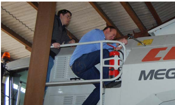
Fig. 53 and Fig. 54: Opening of a grain tank on a combine harvester (Claas Mega 350). Half a turn is required to open the tank. Measurement by means of a hand-held force meter. Left: test subject 1; right: test subject 2
