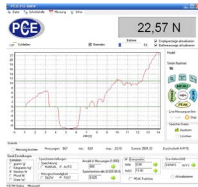
Fig. 43: Software user interface for the PCE-FG 500 hand-held force meter
