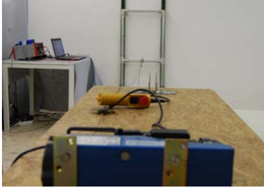
Fig. 154: Disengagement of a ladder. Measurement apparatus with winch
