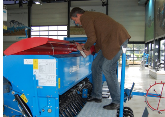
Fig. 108 and Fig. 109: Closing of the seed flap on a seed drill (Lemken Saphir 7). Measurement of the pulling force with a hand-held force meter, force transmission by means of a hose clip, test subject 3 (left) and test subject 4 (right)
