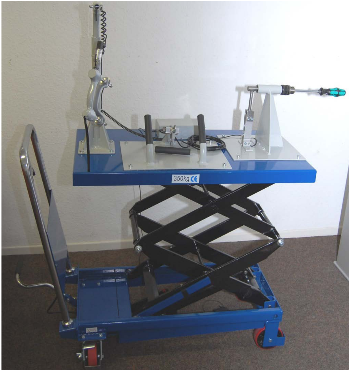
Fig. 59: Mobile force measurement apparatus of the ASER institute for field research. Measurements are possible of hand grip, strain and torsional forces. Mounting of the measurement apparatus on the scissor elevating table enables measurements to be performed in standardized body postures
