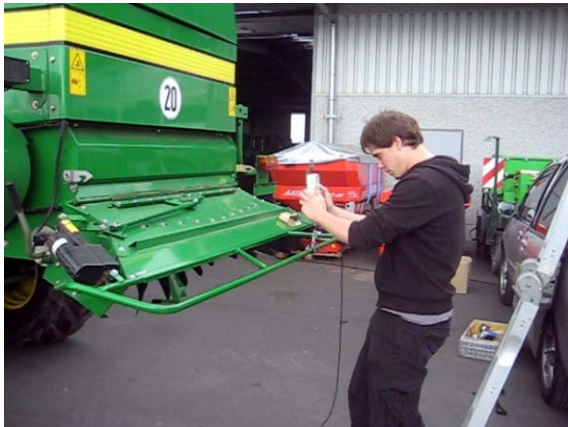
Fig. 102 and Fig. 103: Raising of the chopper on a combine harvester (John Deere T560). Measurement of the pulling force by means of a hand-held force meter; force transmission by means of a hose clip; test subject 2
