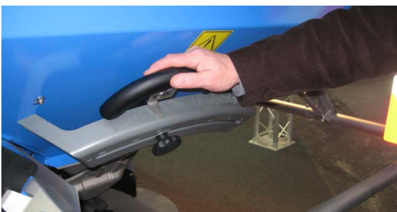
Fig. 35: Angle adjustment with locking screw on a manure spreader (Rabe Adler DSX 36)
