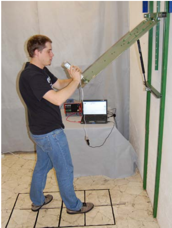
Fig. 140: Closing of a flap. Test subject 2 with hand-held force meter
