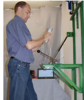
Fig. 134: Operation of a lever. Test subject 5 with hand-held force meter. The meter is held at a 90° angle to the lever
