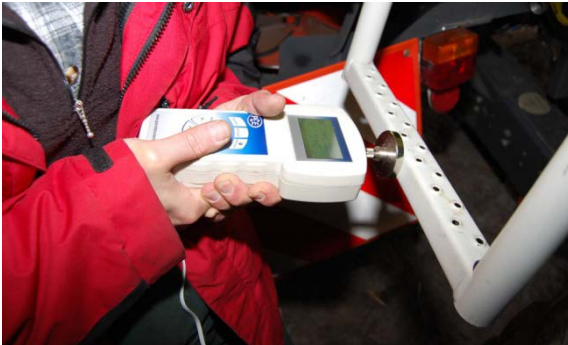
Fig. 114: Engaging the ladder to the grain tank on a combine harvester (Claas Mega 350), test subject 3
