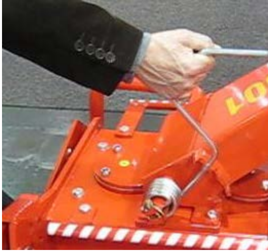
Fig. 74: Lever with handle that is too thin, thus impeding force transmission
