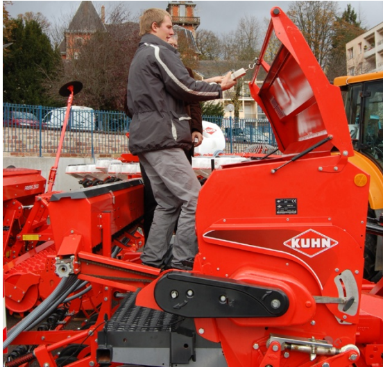
Fig. 111 and Fig. 112: Closing of the seed flap on a seed drill (Kuhn Integra). Measurement of the pulling force with a hand-held force meter, force transmission by means of a hose clip, test subject 5 (left) and test subject 3 (right)
