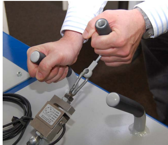
Fig. 61: Measurement of the pulling force
