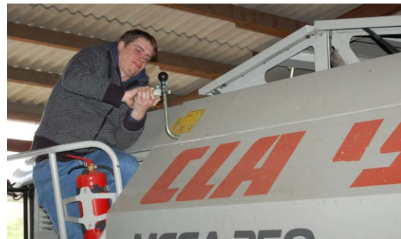
Fig. 53 and Fig. 54: Opening of a grain tank on a combine harvester (Claas Mega 350). Half a turn is required to open the tank. Measurement by means of a hand-held force meter. Left: test subject 1; right: test subject 2
