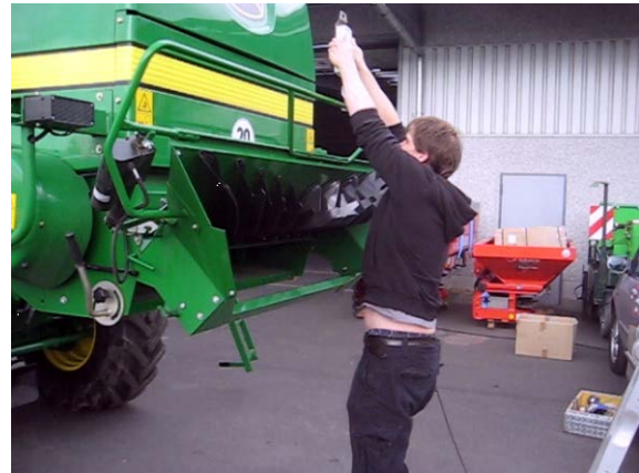
Fig. 102 and Fig. 103: Raising of the chopper on a combine harvester (John Deere T560). Measurement of the pulling force by means of a hand-held force meter; force transmission by means of a hose clip; test subject 2
