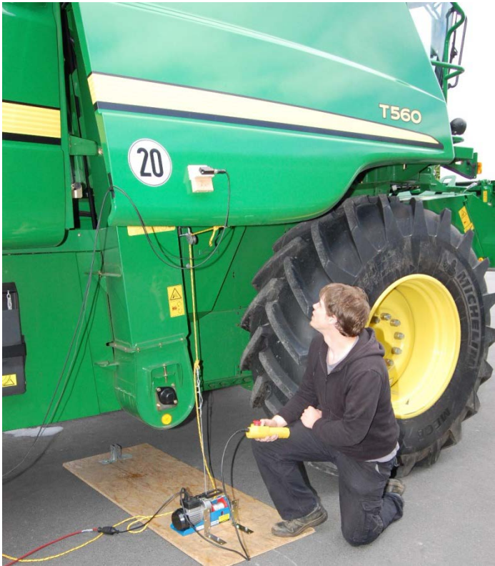
Fig. 100: Closing of the left-hand side flap on a combine harvester (John Deere T560): measurement of the pulling force by means of the complex method
