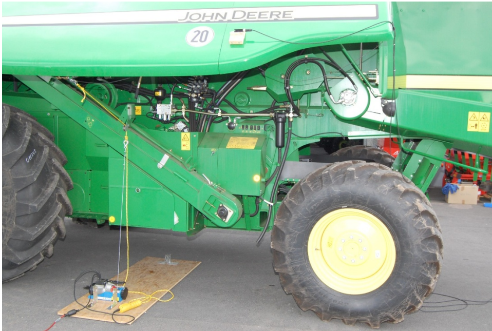
Fig. 95: Closing of the left-hand side flap on a combine harvester (John Deere T560): measurement of the pulling force by means of the complex method
