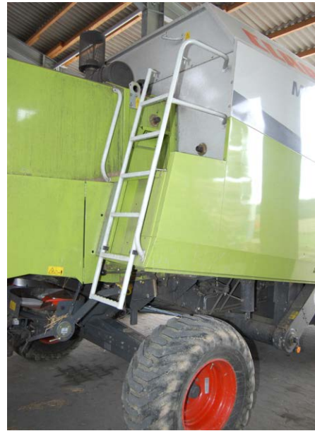
Fig. 28: Ladder to the grain tank on a combine harvester (Claas Mega 350), with engaging arrangement
