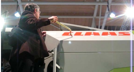
Fig. 11: Opening of a grain tank on a combine harvester (Claas Avero); a full turn is required to open the tank
