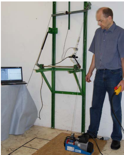
Fig. 56: Operation of a lever. Measurement assembly with winch (automated speed, strain sensor and angle measurement)
