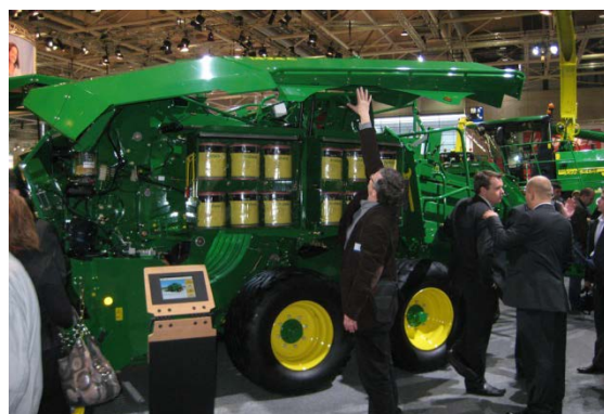
Fig. 22: Side flap on a big baler (John Deere 1424)
