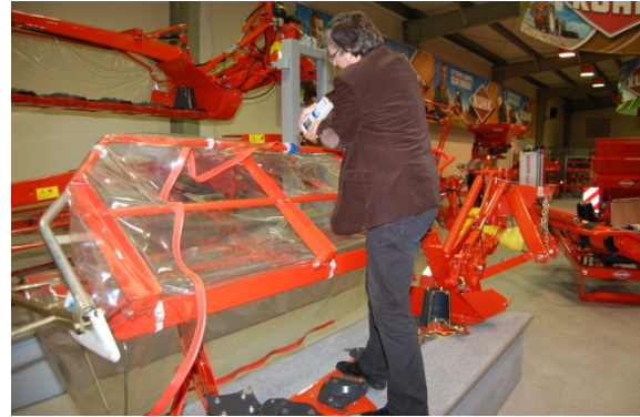
Fig. 105 and Fig. 106: Raising and closing of the cover on a disk mower (Kuhn GMD 600 GII), measurement of the pulling force by means of a hand-held force meter; force transmission by means of a hose clip; test subject 3. For greater clarity, the tarpaulin is transparent
