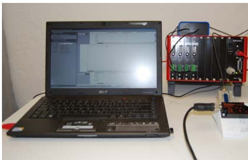
Fig. 44: Force measurement system based upon NextView software with bmcm measurement amplifier
