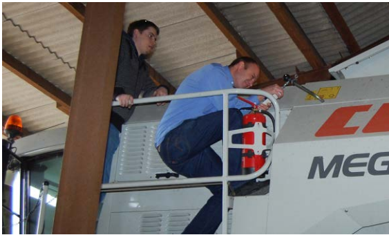
Fig. 76 and Fig. 77: Opening of a grain tank on a combine harvester (Claas Mega 350). Half a turn is required to open the tank. Measurement by means of a hand-held force meter. Left: test subject 1; right: test subject 2
