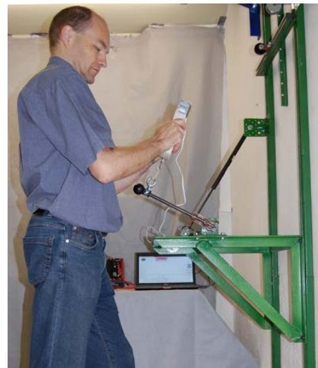
Fig. 57: Operation of a lever. Test subject 5 with hand-held force meter. The meter is held at a 90° angle to the lever
