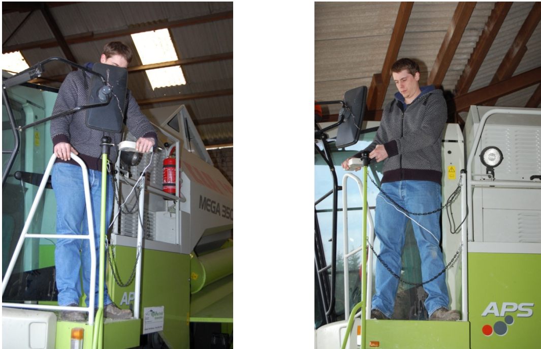
Fig. 127 and Fig. 128: Rotating the ladder to the driver's cab out and in, combine harvester (Claas Mega 350). Measurement with a hand-held force meter, force application point with rope, test subject 2
