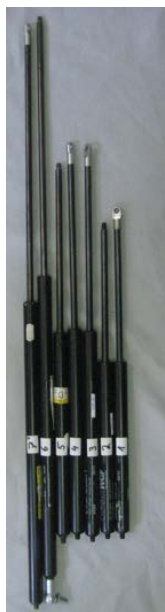
Fig. 138: Gas springs of different lengths and pressures used in the laboratory tests
