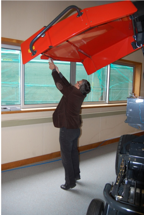
Fig. 89 and Fig. 90: Closing of the side flap on a round baler (Kuhn VB 2190): measurement of the pulling force by means of a hand-held force meter, force transmission via a draw hook on a metal strut, test subject 3. Below an opening angle of approximately 30°, the force of the gas spring is overcome and the flap drops into the engagement mechanism of its own accord
