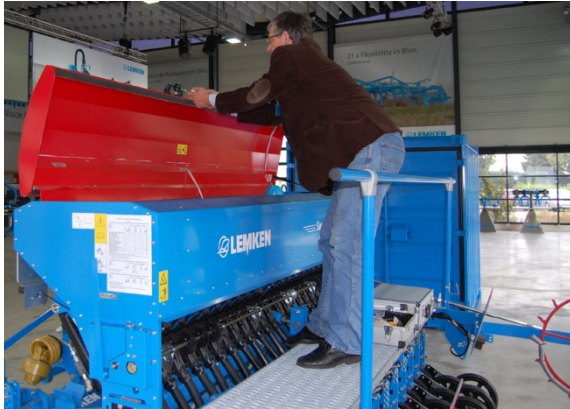
Fig. 108 and Fig. 109: Closing of the seed flap on a seed drill (Lemken Saphir 7). Measurement of the pulling force with a hand-held force meter, force transmission by means of a hose clip, test subject 3 (left) and test subject 4 (right)
