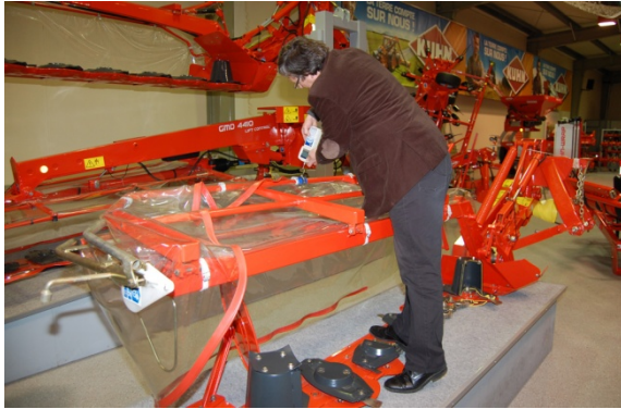
Fig. 105 and Fig. 106: Raising and closing of the cover on a disk mower (Kuhn GMD 600 GII), measurement of the pulling force by means of a hand-held force meter; force transmission by means of a hose clip; test subject 3. For greater clarity, the tarpaulin is transparent
