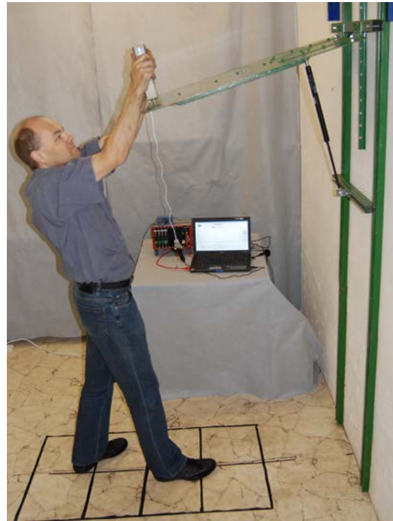
Fig. 141: Closing of a flap. Test subject 5 with hand-held force meter
