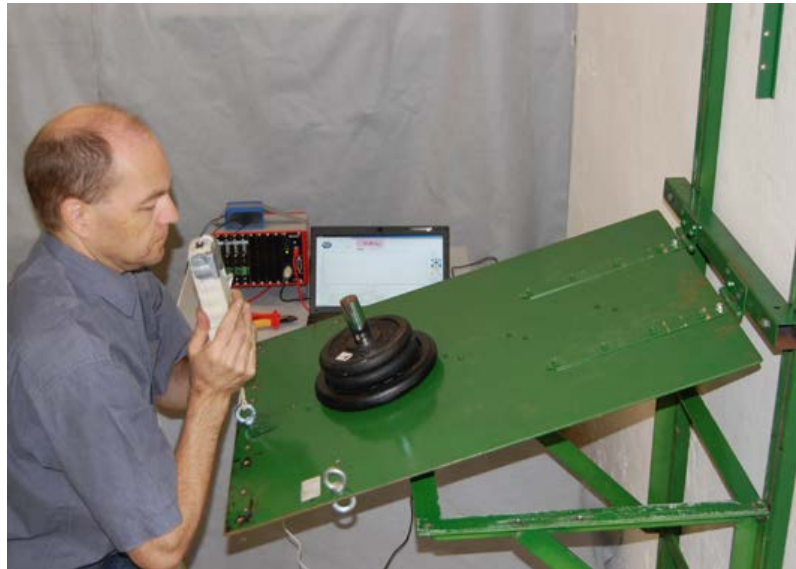
Fig. 149: Raising and lowering of a chopper. Test subject 5 with hand-held force meter
