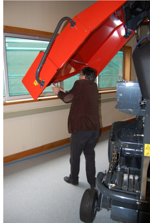
Fig. 89 and Fig. 90: Closing of the side flap on a round baler (Kuhn VB 2190): measurement of the pulling force by means of a hand-held force meter, force transmission via a draw hook on a metal strut, test subject 3. Below an opening angle of approximately 30°, the force of the gas spring is overcome and the flap drops into the engagement mechanism of its own accord
