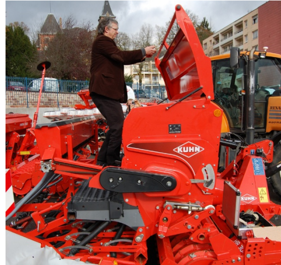
Fig. 111 and Fig. 112: Closing of the seed flap on a seed drill (Kuhn Integra). Measurement of the pulling force with a hand-held force meter, force transmission by means of a hose clip, test subject 5 (left) and test subject 3 (right)
