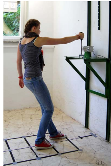
Fig. 65: Measurement arrangement for lever measurements. In this example: measurement at the position X=2, Y=2
