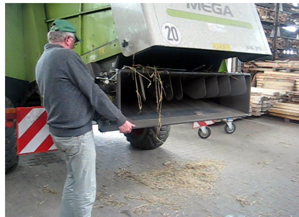
Fig. 26: Manual chopper adjustment on a combine harvester (Claas Mega 350) The chopper is raised with one hand and engaged in position with the other
