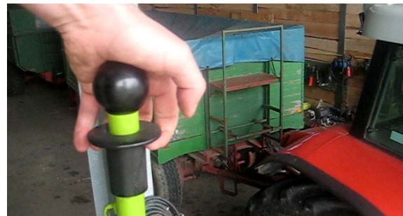
Fig. 34: Swivel-release mechanism on the steps of a combine harvester (Claas Mega 350)
