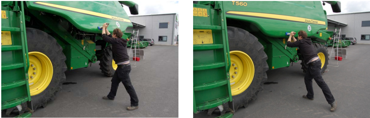
Fig. 92 and Fig. 93: Closing of the left-hand side flap on a combine harvester (John Deere T560): measurement of the pushing force by means of a hand-held force meter, force transmission through a plastic mat to prevent damage to the surface, test subject 2
