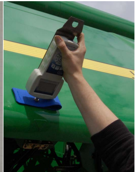
Fig. 52: Use of a rubber mat to prevent damage to paintwork during measurement
