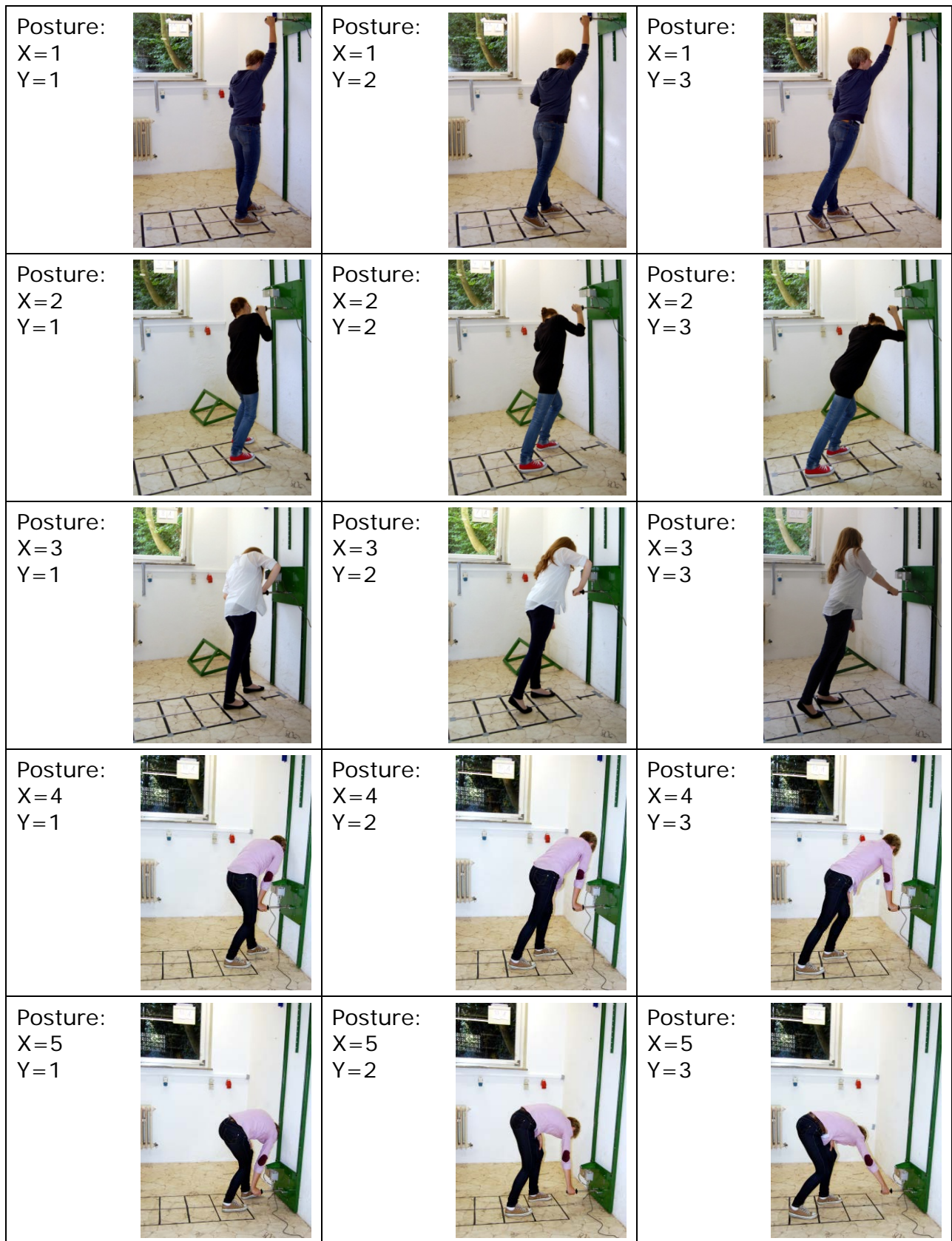
Fig. 159: The 15 body postures, shown with reference to the example of pulling/pushing the lever up/down (direction of force A+ /A-)
